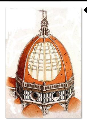
Brunelleschi built the dome out of bricks, due to its light weight compared to stone and easier to form, and with nothing under it during construction. To illustrate his proposed structural plan, he constructed a wooden and brick model with the help of Donatello and Nanni di Banco and still displayed in the Museo dell'Opera del Duomo. The model served as a guide for the craftsmen, but was intentionally incomplete, so as to ensure Brunelleschi's control over the construction.
